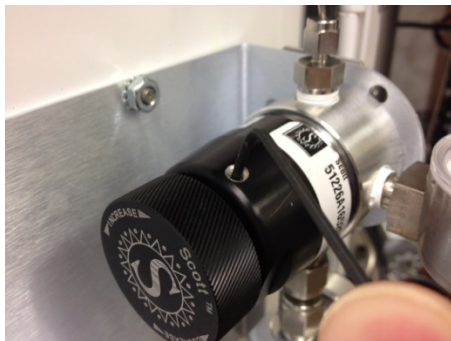
Figure 8: Scott regulator set screw
